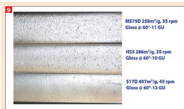
9 Surface roughness of extrudates having similar gloss at 60°.
